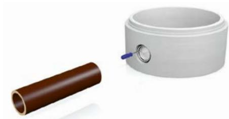
Remove polystyrene from socket.
